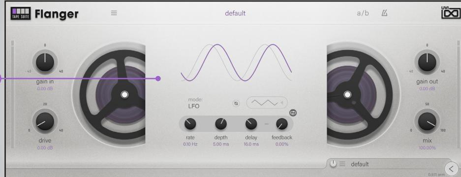
Analog tape flanger featuring through-zero flanging and control in manual or LFO modes (with possible sync to host), for a velvety, organic sound.
